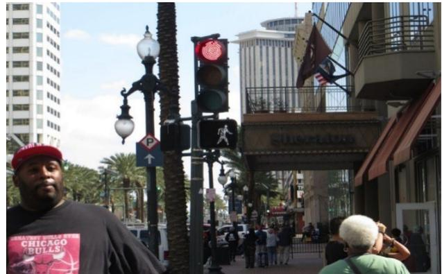
Historically, a standard **walking speed** of 4.0 feet per second has been used to calculate the minimum pedestrian clearance interval for signals. The CAMUTCD provides guidance that a slower walking speed of 3.5 feet per second should be used, and 2.8 feet per second should be considered where pedestrians who are older or who have disabilities routinely use the crosswalk.<sup>10</sup>
