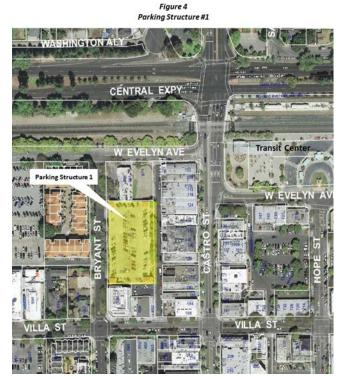
Parking Structure No. 1 is a three-story parking structure, with rooftop parking, with a total of 313 parking stalls, six of which are designated and marked for handicap parking. The structure is constructed of steel-framed concrete, ornamental stucco on exterior, and was constructed in 1989. The current condition of the structure is considered good.
