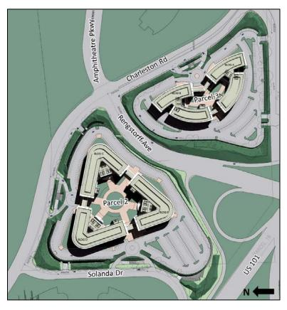
proposed to have two buildings around courtvard totaling 407,000 sq. ft. (at 1.0 FAR) with enclosed skv bridges between buildings and two-levels of parking - one partially underground level and a podium level - on a 9.3acre site. The project result in would the removal of numerous trees, some of which may be heritage trees. The project sites are located at the intersection Charleston Road, North Rengstorff Avenue, and Amphitheatre Parkway immediately north of US 101 freeway.
