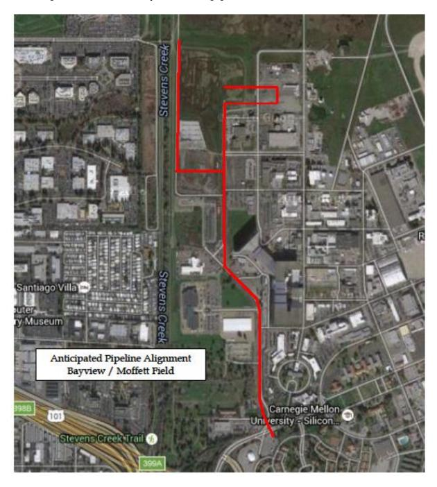
The 2014 feasibility study identified the Middlefield-Ellis-Whisman area as the next priority for expansion of the City's recycled water system (Alternative 2 on Attachment 1). This area can be served by extending the Google-installed system to the edge of Federal property, and then across U.S. 101. The City of Sunnyvale has also expressed interest in connecting to Mountain View's system, which can be accomplished through this expansion.
