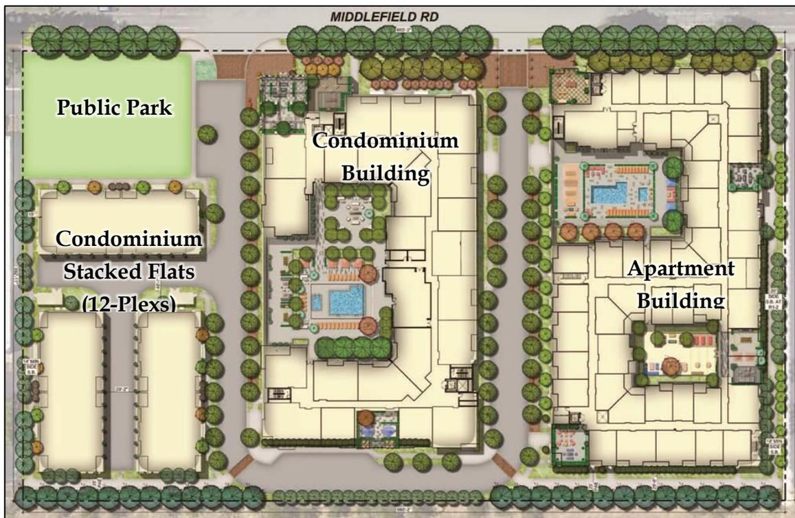
Project site access is proposed from two entrances on Middlefield Road connected by a U-shaped service street with access to the podium parking garages for the apartment and condominium buildings and a set of alleys to individual garages at the stacked flat buildings. Further vehicle, pedestrian, and bicycle circulation is described in the Circulation Section of this report.
