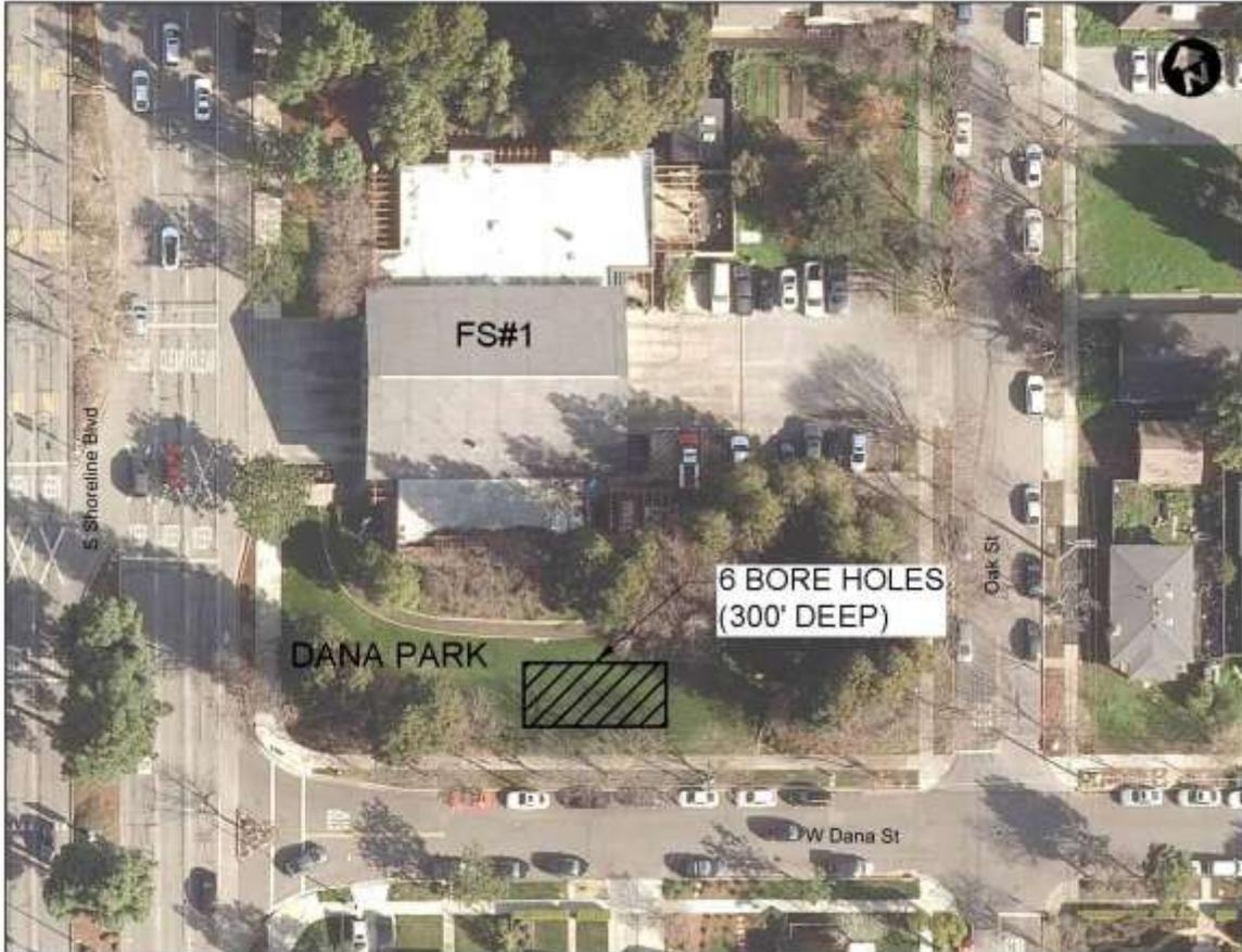
**Figure 1: Fire Station No. 1 Heat Exchange Field**
