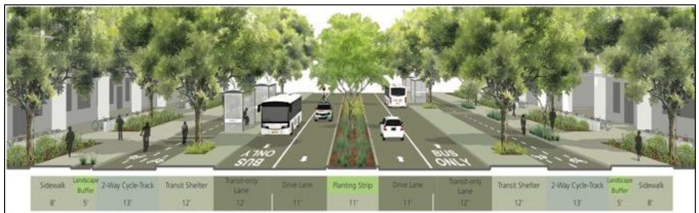
Figure 2: Charleston Transit Boulevard Typical Cross-Section
