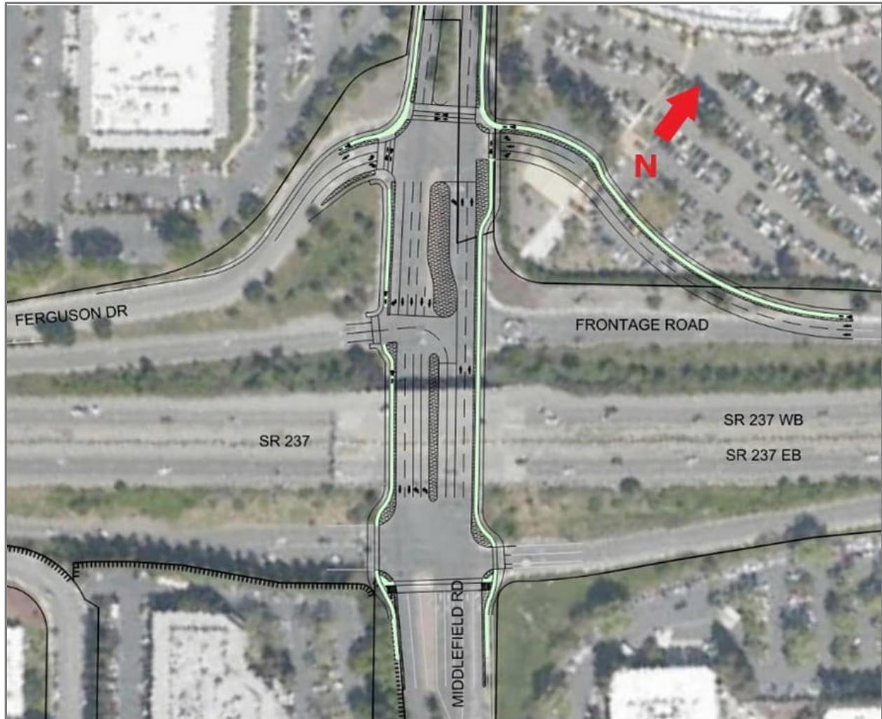
Figure 7 – Alternative 4 – Frontage Road and Ferguson Drive Realignment
