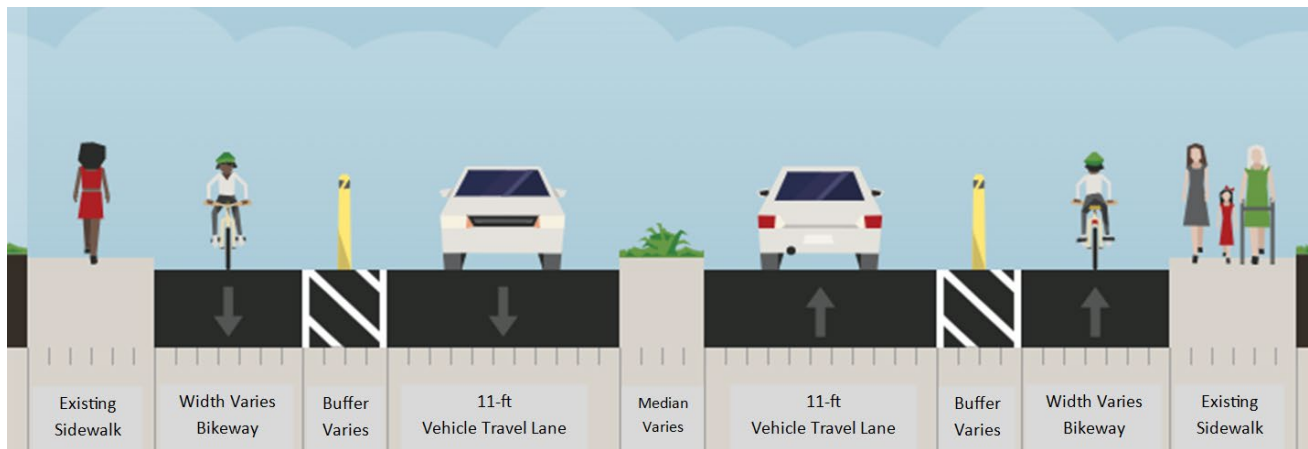
Figure 10: Typical Cross-Section from Miramonte Avenue from Trophy Drive to Marilyn Drive
