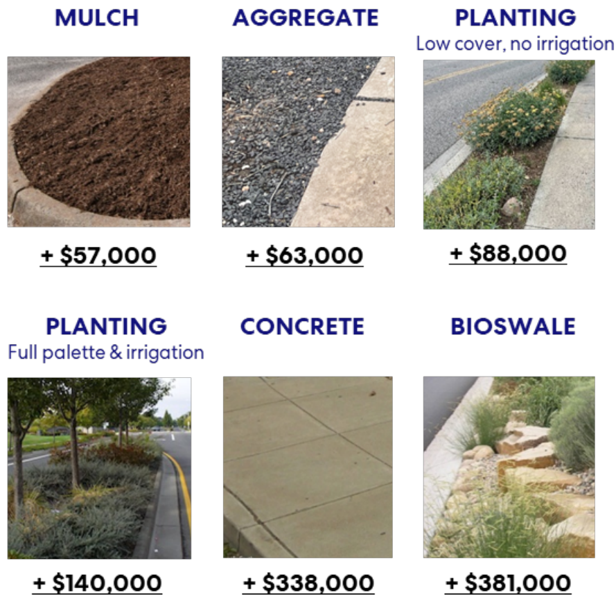
FIGURE 30 ADD-ON COST PER MILE FOR MATERIAL ALTERNATIVES IN REIMAGINED STREETS BEYOND BASE STREET MODIFICATION COST
