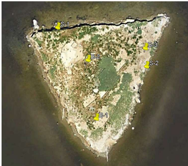
Figure 2-8 Boring and Soil Sample Locations
