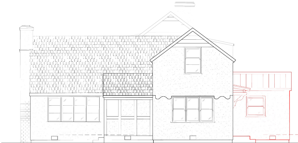
Figure 18. Elevation drawing of the south facade illustrating areas of new construction and alterations in red. Source: "Proposed Remodel For: The Bettman Residence" prepared by Flury Bryant Design Group, Inc. (dated July 16, 2024), Sheet 7. Edited by Page & Turnbull.
