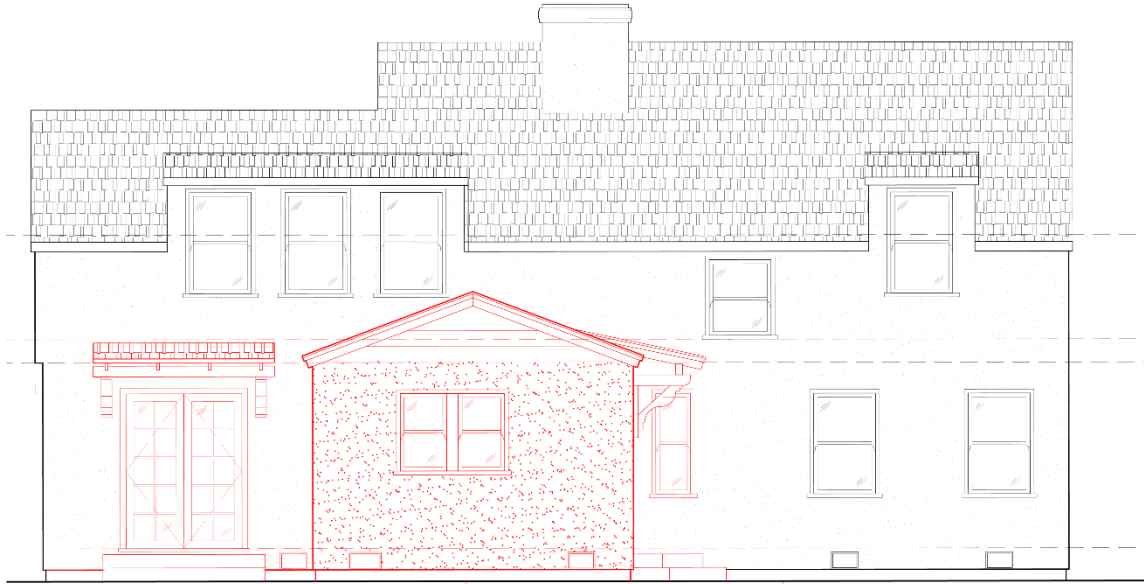
Figure 17. Rear east elevation drawing illustrating areas of new construction and alterations in red. Source: "Proposed Remodel For: The Bettman Residence" prepared by Flury Bryant Design Group, Inc. (dated July 16, 2024), Sheet 7. Edited by Page & Turnbull.
