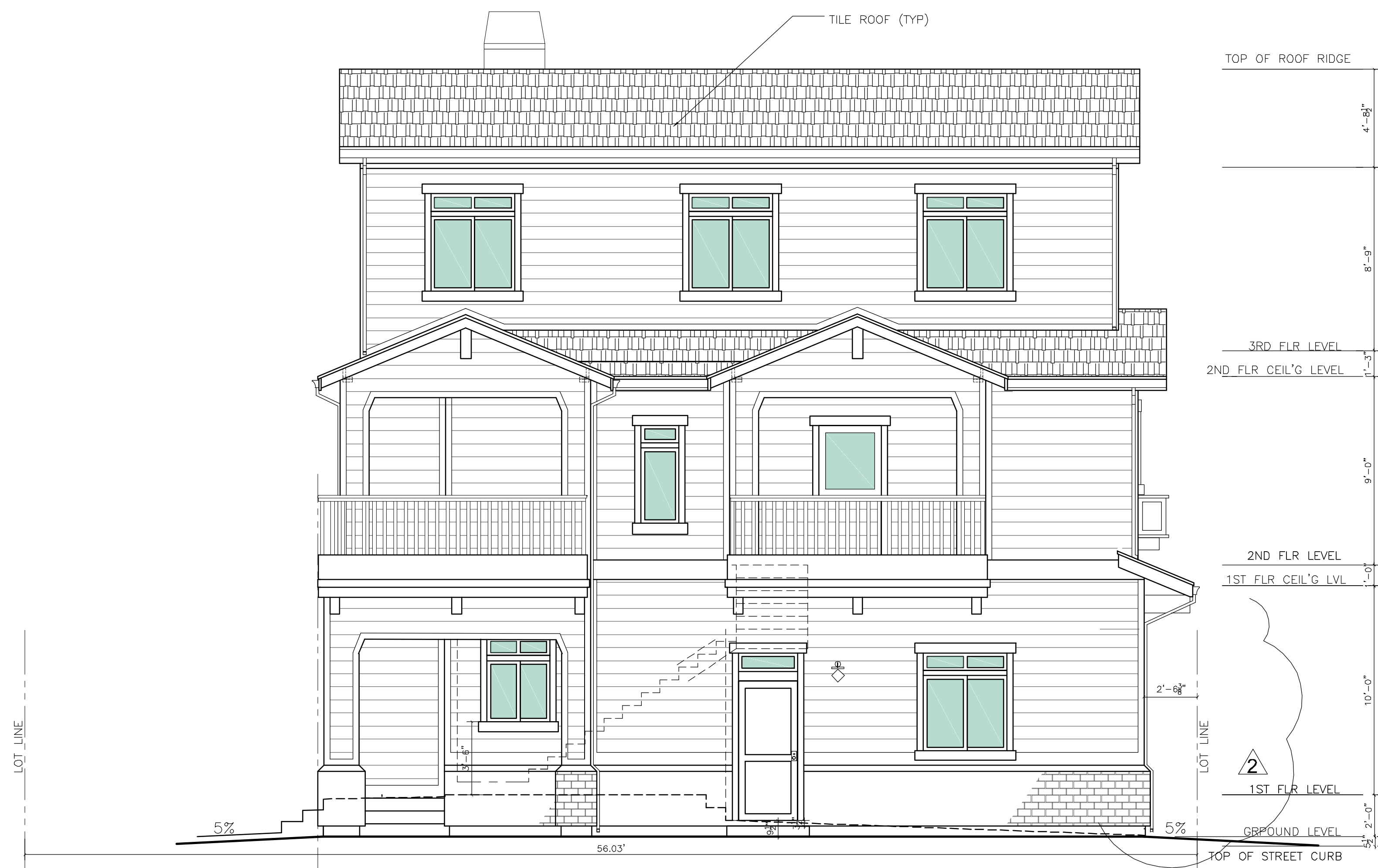
SIDE ELEVATION VIEW "B" SCALE: 1/4"=1'-0" FOR INFORMATION NOT SHOWN, SEE ELEVATION "A"
