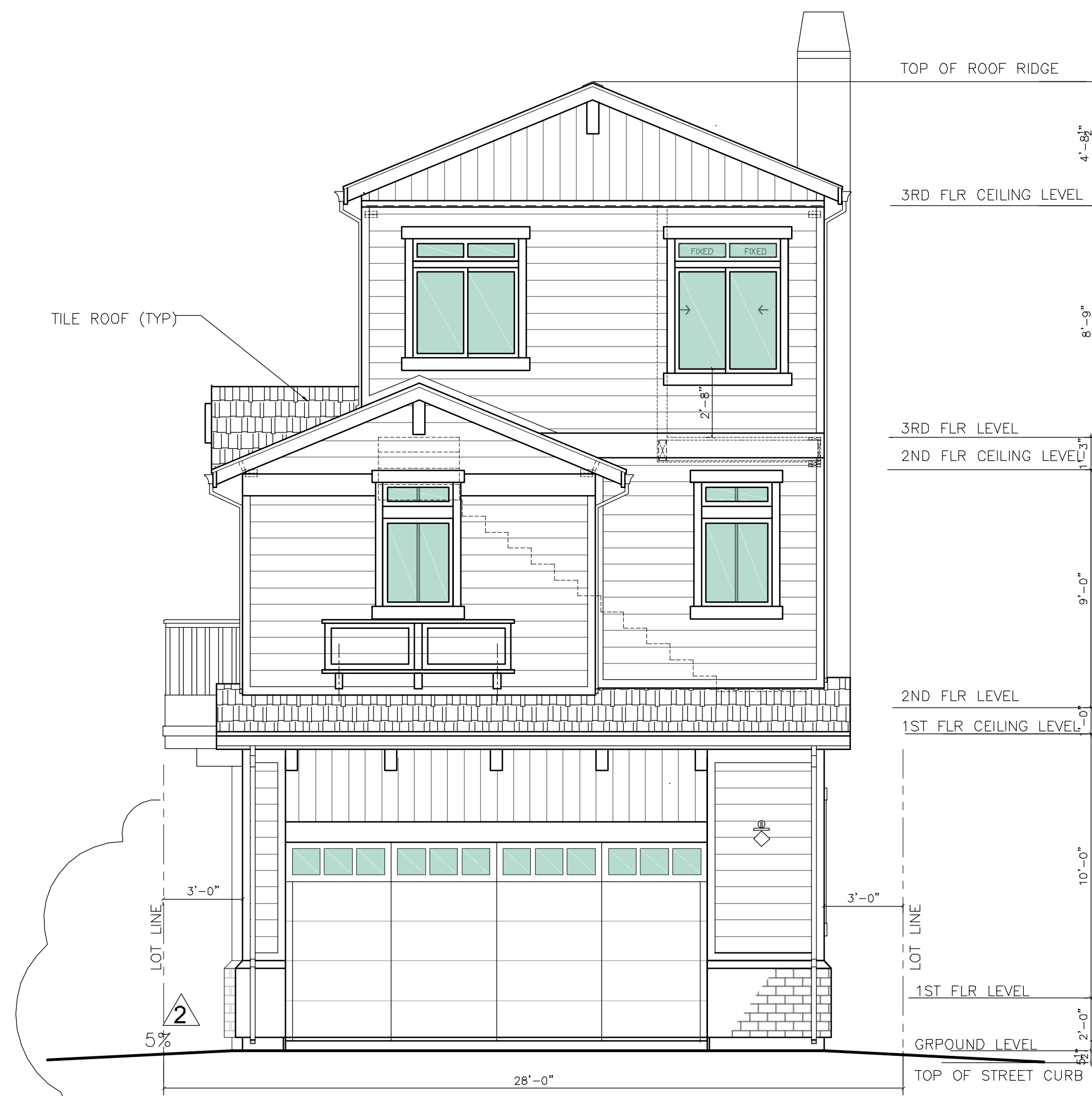
REAR ELEVATION VIEW "C" SCALE: 1/4"=1'-0" FOR INFORMATION NOT SHOWN, SEE ELEVATION "A"
