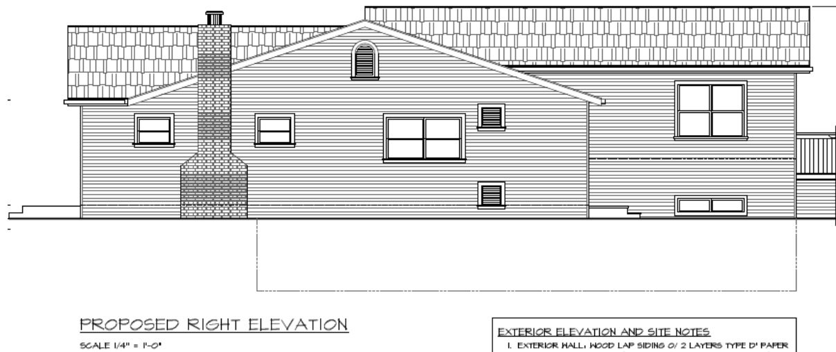
Figure 13. East (right) elevations, showing the proposed addition, removed brick sidewall, and removed internal chimney. Source: "Single Family House", by Better Built Builders, (February 2, 2025), Sheet A-7.
