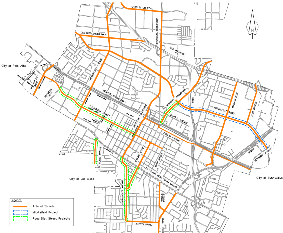
Figure 3: Implemented and Planned Road Diets
