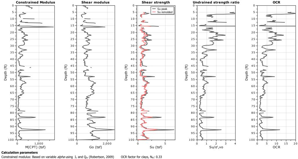
Go: Based on variable *alpha* using  $I_c$  (Robertson, 2009) Undrained shear strength cone factor for clays, N<sub>kt</sub>: 14
