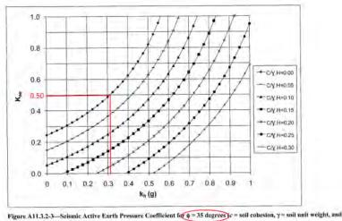
Figure A11.3.2-3—Seismic Active Earth Pressure Coefficient for  $\phi = 35$  degrees to e = soil cohesion,  $\gamma = soil unit weight = retaining wall height)$
