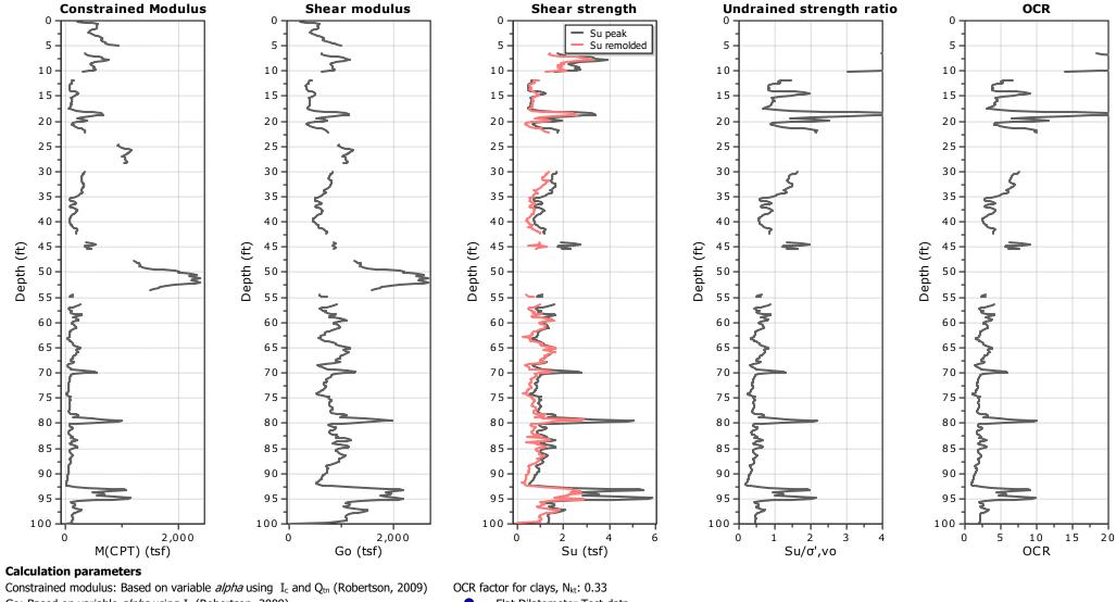
Go: Based on variable *alpha* using I<sub>c</sub> (Robertson, 2009) Undrained shear strength cone factor for clays, Nkt: 14
