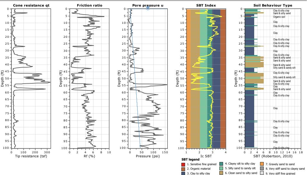
Surface Elevation: 0.00 ft Coords: X:0.00, Y:0.00 Cone Type: Cone Operator: Soil Behaviour Type
