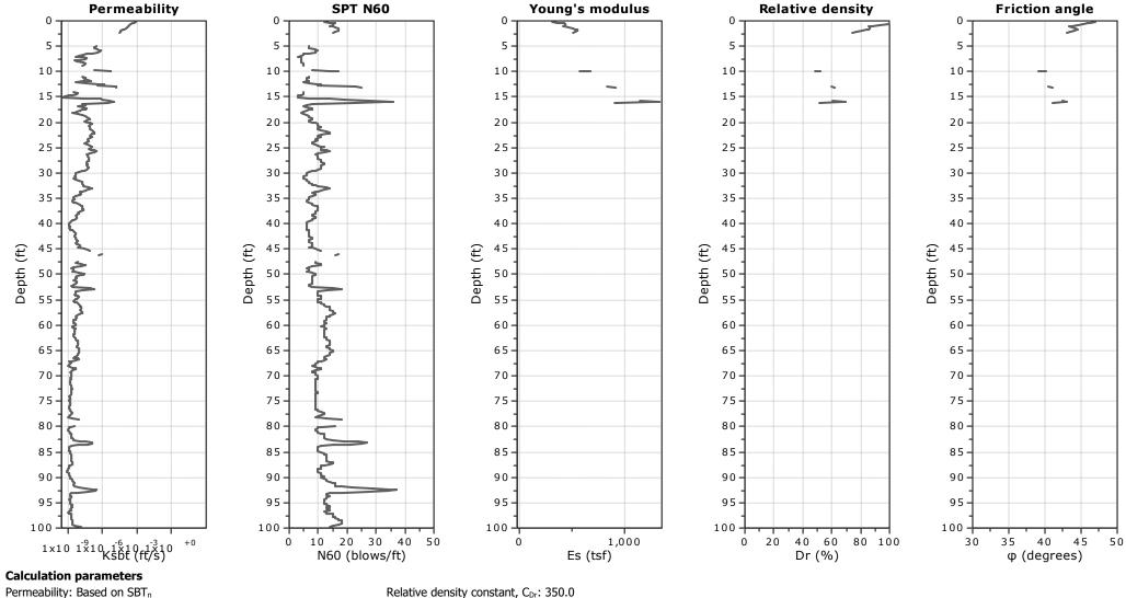
SPT  $N_{60}$ : Based on I<sub>c</sub> and q<sub>t</sub>
