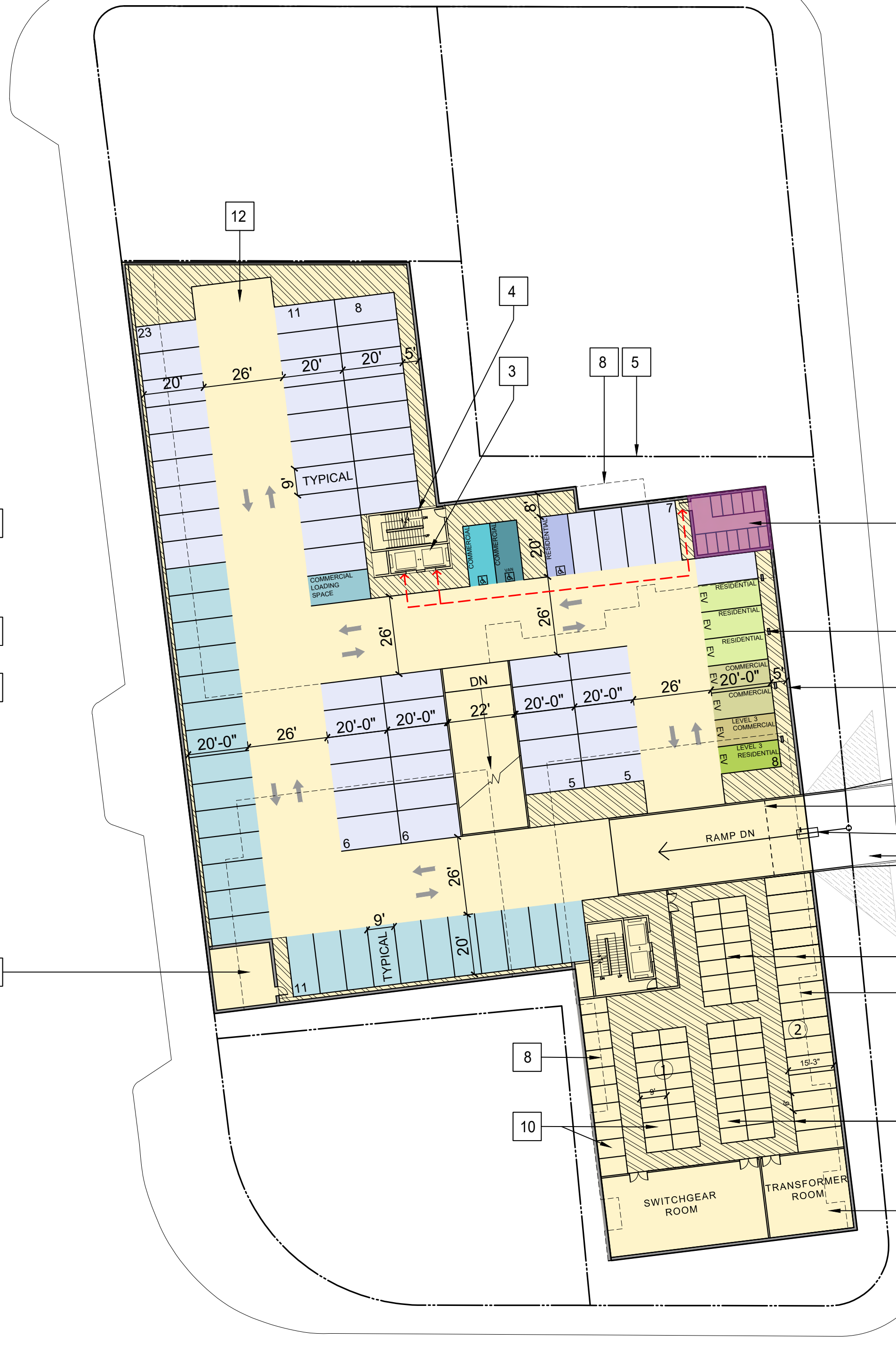
1 BASEMENT LEVEL B1 90 STALLS 48,020 SF 1"=30'-0"
