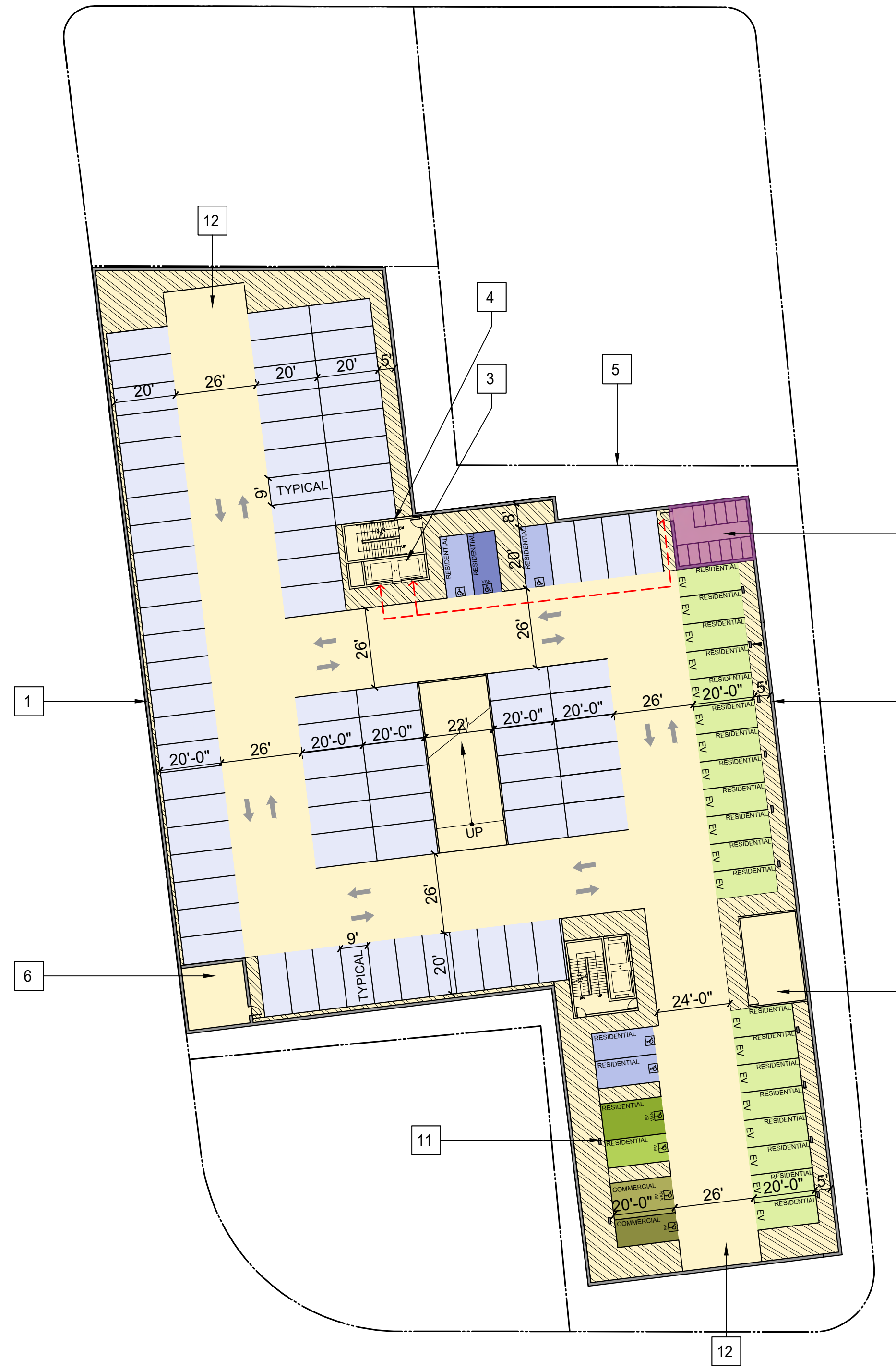
2 BASEMENT LEVEL B2 110 STALLS 48,020 SF 1"=30'-0"
