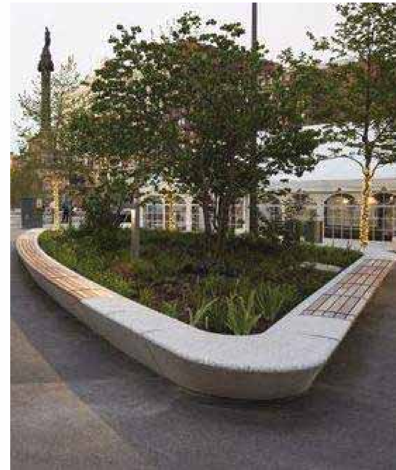
Groundfloor Conc. Planter w/ Wood Top 18"H. Walls (Above Grade) Custom Built
