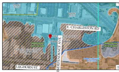
FEMA FLOOD ZONE MAP The project site is located in FEMA Special Flood Hazard Zone AE (EL 11).
