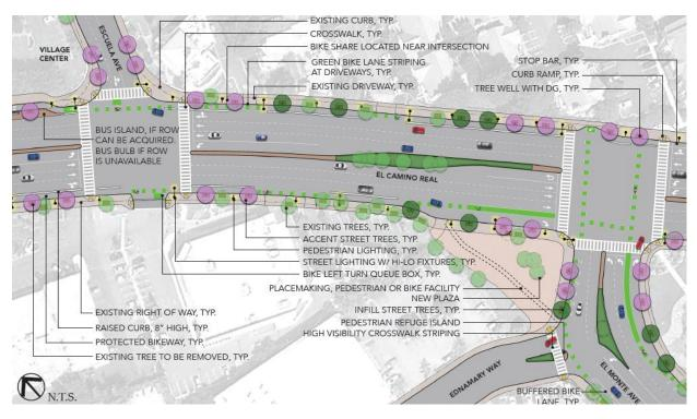
Figure 2: Design Concept for El Monte Avenue/El Camino Real Intersection from El Camino Real Streetscape Plan
