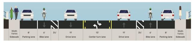
Figure 1: Example Cross Section for Road Diet
