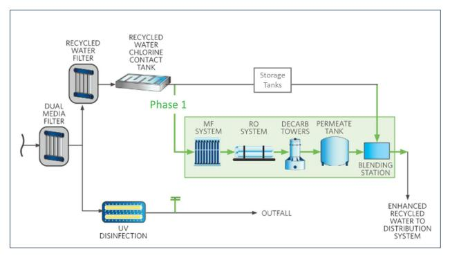
Figure 2: Enhanced Recycled Water Process Flow Diagram
