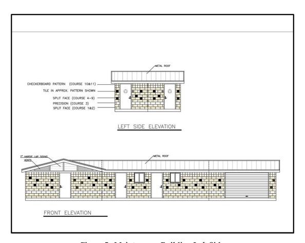
Figure 5: Maintenance Building Left Side
